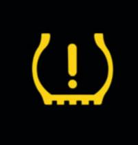
In the event of a change in air pressure, the **flat tyre indicator** symbol appears in the display of the multifunction computer, advising the driver to rectify the situation.
