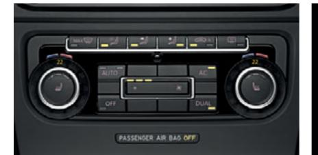
The **2Zone electronic climate control with automatic air recirculation system** features dual zone temperature control for the driver and front passenger, allowing each to select their individually preferred temperature.
