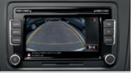
A **rear-view camera**, integrated behind the Volkswagen badge on the rear tailgate provides a clear view to the rear of your vehicle, transmitting an undistorted live image to your radio or navigation system display, enabling you to manoeuvre quickly and easily into the most difficult parking space.
