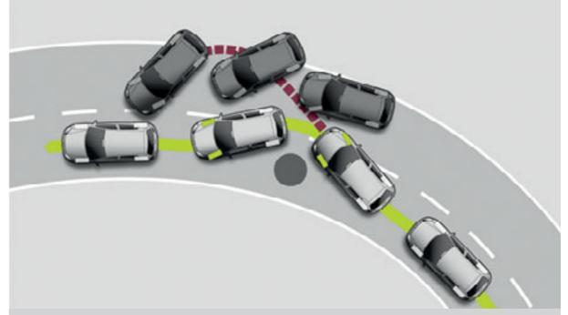
The Electronic Stabilisation Programme (ESP) recognises critical driving situations and reacts in milliseconds by targeting brake and management systems, controlling the speed of individual wheels and helping to bring the vehicle under control. As a result the vehicle achieves maximum directional stability.
