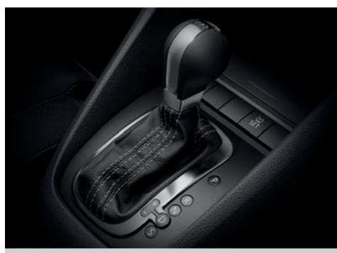
The **dual-clutch Direct Shift Gearbox (DSG)** represents a milestone in the development of the latest gearbox technology. This innovative automatic transmission shifts smoothly and imperceptibly into the pre-selected next gear within a split second, so not only is this six speed gearbox very dynamic, its level of efficiency is almost as economical as its manual counterpart.
