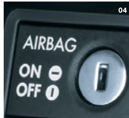
04 The front passenger airbag can be deactivated, to allow the use of a rear facing child seat, by the simple turn of a key.
