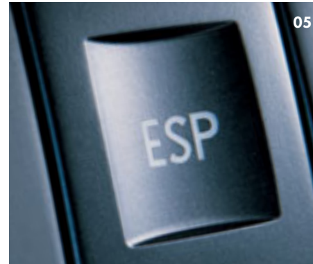
05 In a potentially dangerous situation, the Electronic Stabilisation Programme (ESP) will intervene to diffuse the problem. Through the brake and engine management systems, it will specifically slow down individual wheels for greater stability. However, this enhanced system should not lead to carelessness, because ESP cannot defy the laws of physics. In conjunction with ESP, two other systems are in force to provide improved roadholding and safety. They are Electronic Differential Lock (EDL) and Traction Control (ASR) – a formidable combination to help the vehicle's stability and grip on poor or wet surfaces.
