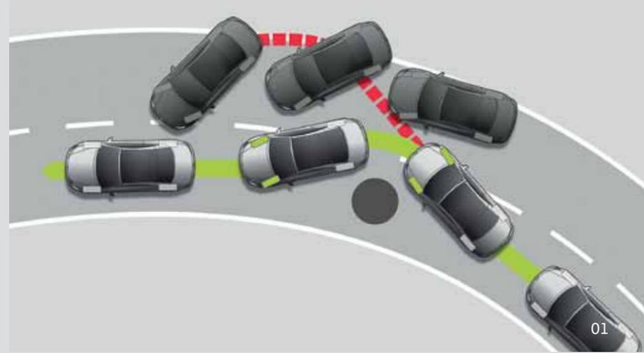
01 The **ESP (Electronic Stabilisation Programme)** recognises critical driving situations and reacts in milliseconds by targeting brake and management systems, controlling the speed of individual wheels and helping to bring the vehicle under control. As a result, the vehicle achieves maximum directional stability. However, a careful driving style is essential, as even ESP cannot extend beyond the laws of physics.
