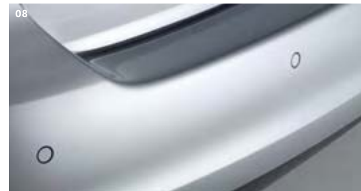
08 The parking sensor emits an audible beep when reversing, as objects behind get closer the time between beeps shortens allowing confident parking every time. Also the passenger's mirror has a reverse activated kerb-view adjustment. Optional on all models.
