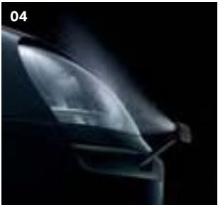
04 The Winter pack offers comfort and safety during the coldest months. The Winter pack includes electrically heated front seats, heated windscreen washer jets, headlight washers and a low washer fluid level warning light. Optional on GT Sport and R32 models.
