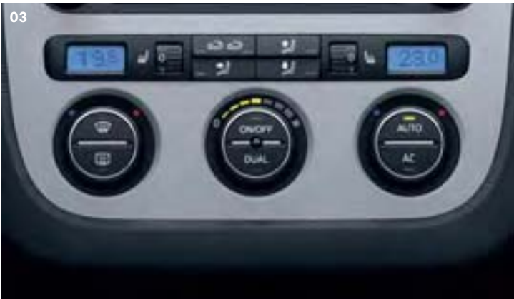
03 The 2Zone electronic climate control is fully automatic to retain a precise internal temperature. It also benefits from a twin zone setting that allows the driver and front passenger up to 4°C difference in their chosen temperature settings. Even the glovebox is chilled should you be carrying snacks on your journey. Standard on R32 and optional on Match, BlueMotion Match and GT Sport.
