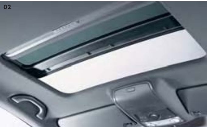
02 The tilt and slide electric glass sunroof is extremely easy to use. Simply turn the automatic function to your desired setting. It also includes a sunblind for added comfort. Optional on Match, BlueMotion Match, GT Sport and R32 models.
