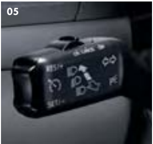
05 Cruise control can be set at speeds over 19 mph to maintain a constant speed. So even on long journeys you can have a high degree of relaxation. Standard on Match, BlueMotion Match and optional on all other models.
