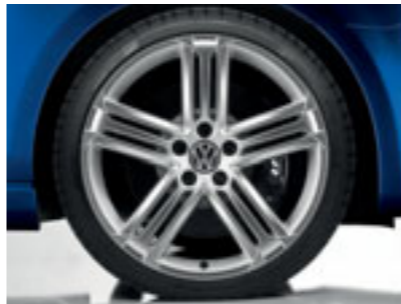
‘Talladega’ 8J x 19 light alloy wheels with 235/35 R19 tyres, includes black headlight surrounds. Optional on R models.
