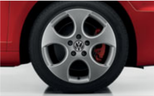
Standard 7½J x 17 'Monza' alloy wheels with 225/45 R17 low profile tyres give the Golf GTI its purposeful image, the distinctive five spoke design revealing the red brake calipers beneath.
