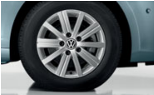
‘Wellington’ 6½J x 15 light alloy wheels with 195/65 R15 low rolling resistance tyres help to reduce the BlueMotion’s fuel consumption.
