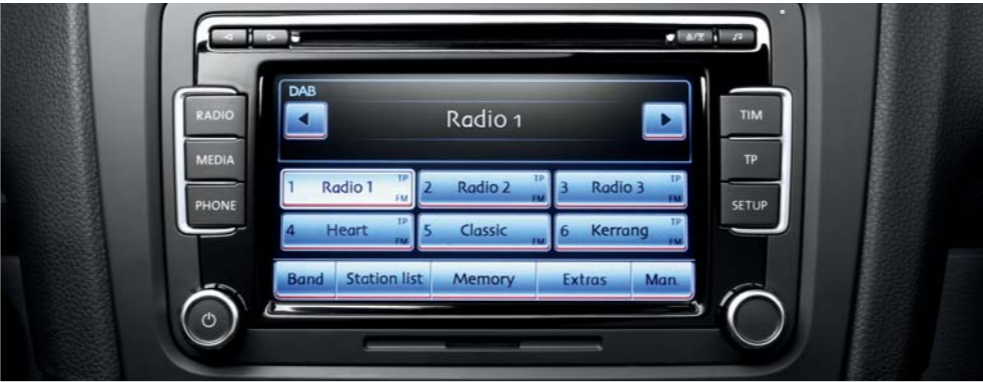
The RCD 510 touch-screen DAB digital radio/dash-mounted MP3 compatible six CD autochanger features a large 6½ inch colour display, with intuitive menu navigation and touch-screen operation. It also features an AUX-in socket for connection to an external multimedia source (e.g. iPod or MP3 player) and an SD memory card slot.
