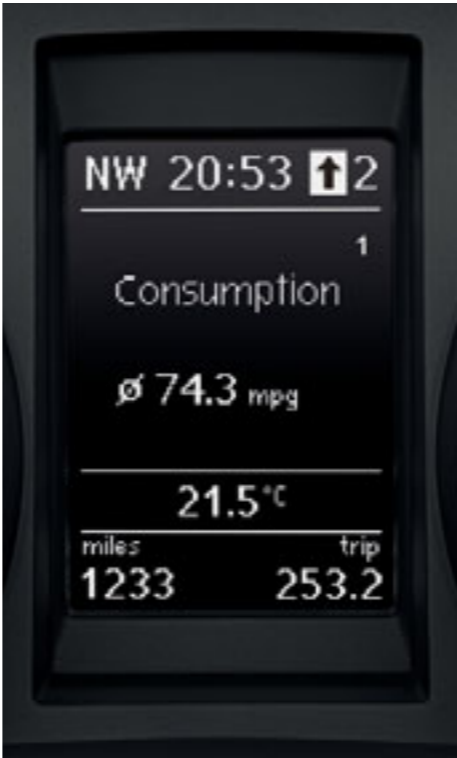
The multifunction computer (Highline) provides useful statistics about your journey, such as exterior temperature, average and current fuel consumption, average speed and estimated distance to refuelling. It also includes a visual gear change recommendation for optimum fuel consumption.
