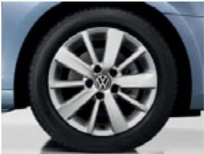
‘Croft’ 6½J x 16 light alloy wheels with 205/55 R16 tyres. Standard on Match and Match BlueMotion Technology models. Please note: Match BlueMotion Technology models are fitted with 205/55 R16 low rolling resistance tyres.
