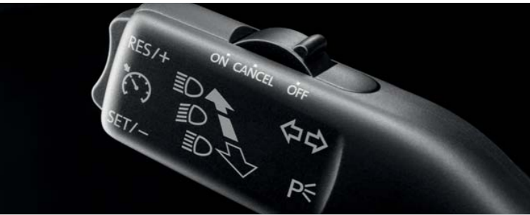
At speeds of over 19 mph, cruise control keeps your selected speed constant, enabling you to relax on longer journeys, without having to keep an eye on your speedometer.
