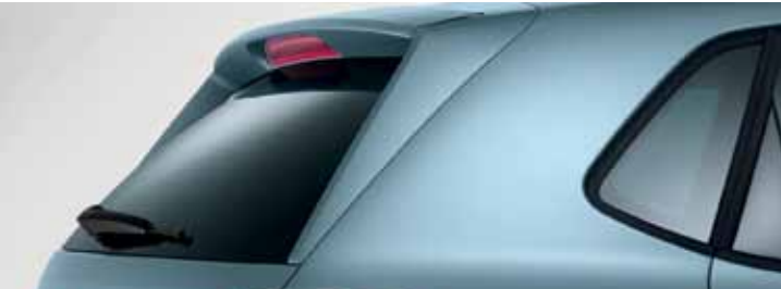
The rear spoiler not only enhances the BlueMotion's dynamic lines but also helps to reduce the vehicle's air resistance, and in turn reduces fuel consumption.
