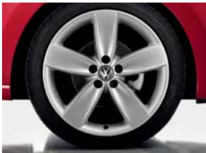
'Boavista' 7J x 17 inch alloy wheels with 215/40 R17 tyres are eye-catching and stylish, and are fitted with anti-theft wheel bolts. Optional on SEL models.
