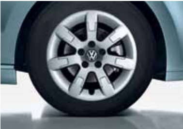
'Greenland' 5½J x 15 light alloy wheels with 185/60 R15 low rolling resistance tyres help to reduce the BlueMotion's fuel consumption.
