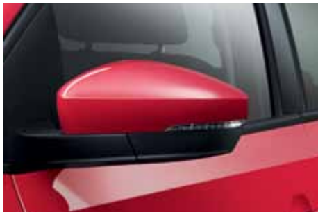
The electrically heated and adjustable body-coloured door mirrors with integrated indicators enhance the exterior of the Polo and can be easily operated from the comfort of the driver's seat.
