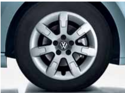
'Greenland' 5½J x 15 light alloy wheels with 185/60 R15 low rolling resistance tyres help to reduce the BlueMotion's fuel consumption. Standard on BlueMotion models.
