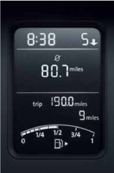
The multifunction computer (Midline) provides useful statistics about your journey, such as exterior temperature, average and current fuel consumption, average speed and estimated distance to refuelling. It also includes a visual gear change recommendation for optimum fuel consumption.
