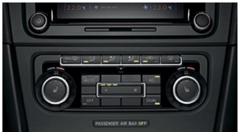
The newly designed 2Zone electronic climate control with automatic air recirculation system features dual zone temperature control for the driver and front passenger, enabling each to select their individually preferred temperature.
