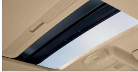
The **tilt and slide electric glass sunroof** is extremely easy to use. Simply turn the automatic function to your desired setting. It also includes a sunblind for added comfort. Optional on all models.
