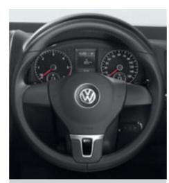
The multifunction leather trimmed steering wheel allows control of the multifunction computer and radio without taking your hands off the wheel. Optional on SE and Sport models.
