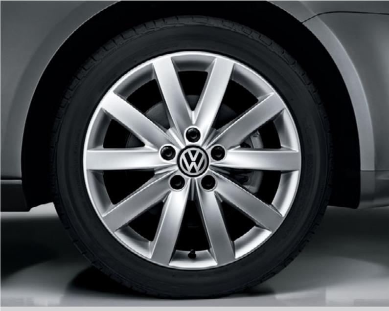
'Porto' design 7J x 17 alloy wheels with 225/45 R17 tyres and anti-theft wheel bolts. Optional on all models. On S and SE models this option includes a temporary steel spare wheel.
