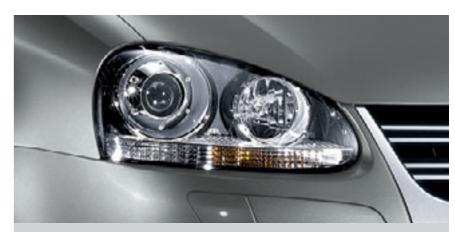
Gas discharge (Xenon) dipped beam headlights with automatic range adjustment improve visibility and the headlight washer system ensure they stay clean. Optional on all models.
