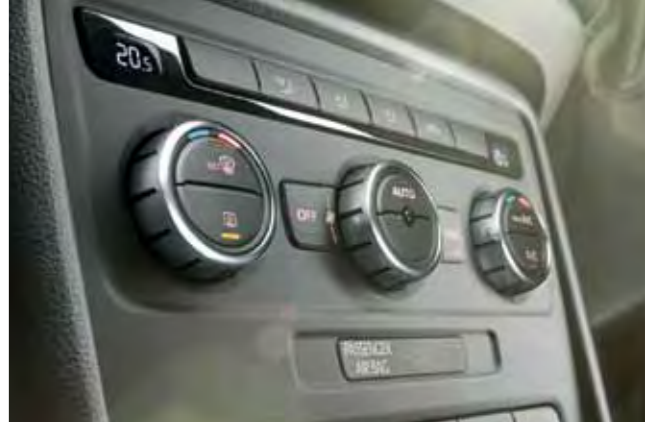
2Zone electronic climate control air conditioning controls the temperature electronically and divides the interior into two different climate zones, enabling the driver and front passenger to adjust the temperature, air supply and distribution to suit their individual preference.
