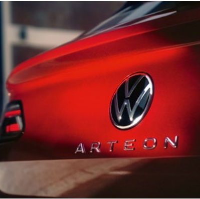
02 New LED tinted tail light clusters with dynamic sequential indicator function and chrome-effect trapezoid dummy exhaust tailpipe surrounds emphasise the new Arteon's striking rear design. Standard on Elegance and R-Line models.
