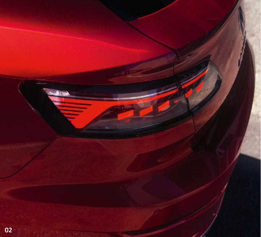
02 New LED tinted tail light clusters with dynamic sequential indicator function and chrome-effect trapezoid dummy exhaust tailpipe surrounds emphasise the new Arteon's striking rear design. Standard on Elegance and R-Line models.
