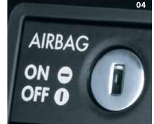
**04** The front passenger airbag can be deactivated, to allow the use of a rear facing child seat, by the simple turn of a key.
