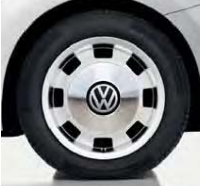
17 inch ‘Orbit’ alloy wheels with 215/55 R17 tyres, chrome effect rims and anti-theft wheel bolts. Standard on Design.
