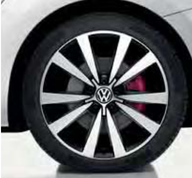
19 inch ‘Tornado’ alloy wheels with 235/40 R19 tyres and anti-theft wheel bolts. Standard on Turbo Black and Turbo Silver, and optional on Sport 2.0 TSI 200 PS models.
