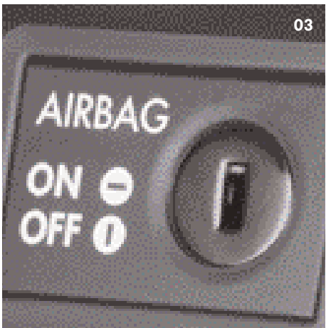
03 The front passenger airbag can be deactivated, to allow the use of a rear facing child seat, by the simple turn of a key.
