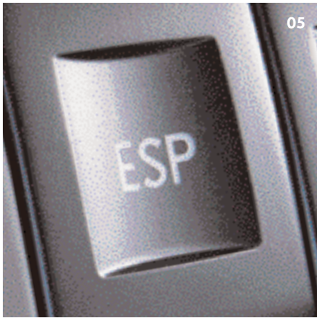
05 In a potentially dangerous situation, the Electronic Stabilisation Programme (ESP) will intervene to diffuse the problem. Through the brake and engine management systems, it will specifically slow down individual wheels for greater stability. However, this enhanced system should not lead to carelessness, because ESP cannot defy the laws of physics. In conjunction with ESP, two other systems are in force to provide improved roadholding and safety. They are Electronic Differential Lock (EDL) and Traction Control (ASR) – a formidable combination to help the vehicle’s stability and grip on poor or wet surfaces.
