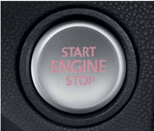
The Keyless entry system enables you to enter and exit your vehicle without taking the key out of your pocket. Once inside, as long as you have the key on you, the engine can be started without inserting the key in the ignition by simply pressing a button in the centre console. Optional on all models except Beetle and Beetle Cabriolet.
