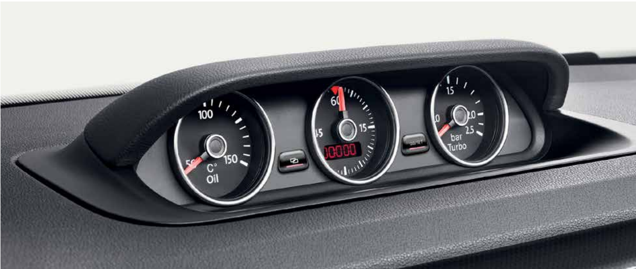
The three dial 'Sport' instrument panel on the dashboard is a particularly distinctive feature showing information about oil temperature and turbocharger boost, as well as the multifunctional stopwatch that can measure the journey time and time stopped. Standard on Sport, Beetle Turbo Black and Turbo Silver, and optional on all Design models.
