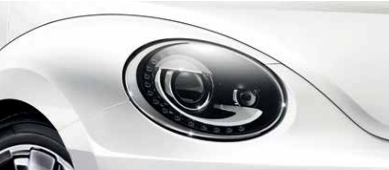
Bi-xenon headlights including range adjustment and LED daytime running lights make it unmistakably Volkswagen. Optional on all models.
