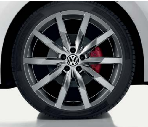
20 inch 'Monterrey' alloy wheels with 235/35 R20 tyres and anti-theft wheel bolts. 1.4 litre TSI 150 PS and 2.0 litre TDI 150 PS engines also include optional sports suspension. [SP] Image shown is Beetle Sport 2.0 litre TSI 220 PS.
