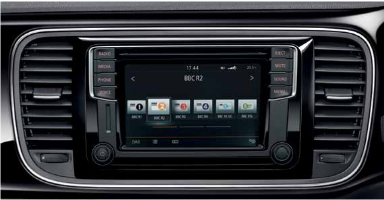
The Composition Media system is equipped with a 6.5 inch colour touch-screen, DAB digital radio receiver, dash-mounted single CD player, SD card reader, and 8 speakers front and rear with 4 x 20 watt output. It facilitates music playback from MP3, WMA and AAC files and features title and compatible cover art display. There is also SMS functionality which allows you to read, compose and send SMS messages using the touch-screen display (compatible Android smartphones only). An MDI (Multi Device Interface) via USB connection for connectivity to an external multimedia source. You can also stream music to the vehicle's audio system via Bluetooth connection 1 , should you wish, from a compatible device. Finally, the Think Blue. Trainer. – provides driver tips and journey analysis to help promote economical driving. Optional on Beetle and Beetle Cabriolet and standard on all other models.
