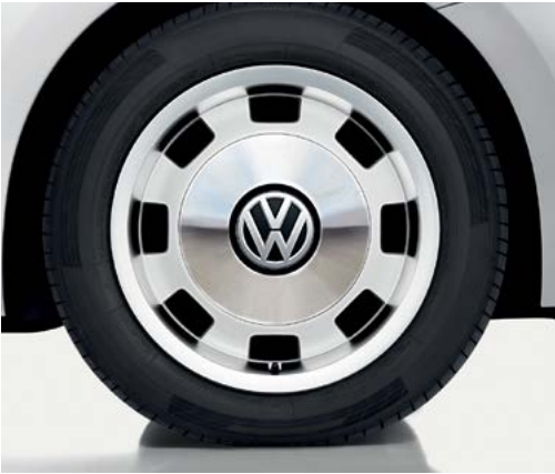
17 inch 'Orbit' alloy wheels with 215/55 R17 tyres, chrome effect rims and anti-theft wheel bolts. [D]
