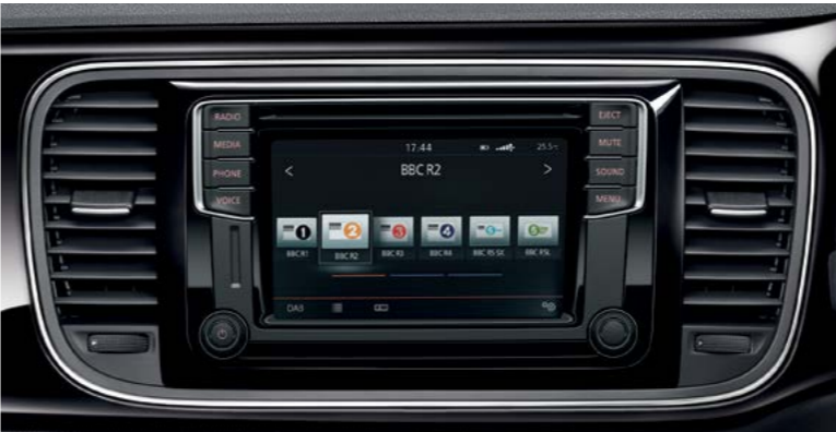
The Composition Media system is equipped with a 6.5 inch colour touch-screen, DAB digital radio receiver, dash-mounted single CD player, SD card reader, and 8 speakers front and rear with 4 x 20 watt output. It facilitates music playback from MP3, WMA and AAC files and features title and compatible cover art display. There is also SMS functionality which allows you to read, compose and send SMS messages using the touch-screen display (compatible Android smartphones only). An MDI (Multi Device Interface) via USB connection for connectivity to an external multimedia source. You can also stream music to the vehicle's audio system via Bluetooth connection 1 , should you wish, from a compatible device. Finally, the Think Blue. Trainer. – provides driver tips and journey analysis to help promote more economical driving. Optional on Beetle and Beetle Cabriolet and standard on all other models.
