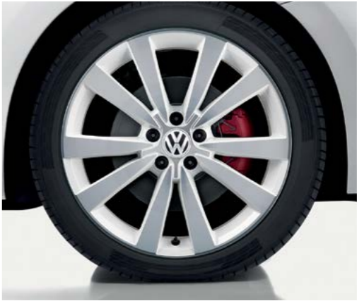
19 inch 'Tornado White' alloy wheels with 235/40 R19 tyres and anti-theft wheel bolts. SP Image shown is Beetle Sport 2.0 litre TSI 220 PS.
