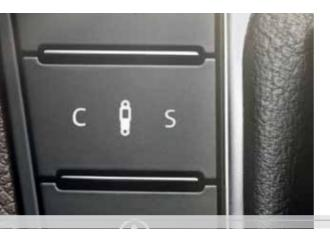
ADAPTIVE CHASSIS CONTROL (ACC) gives you the choice to select Sport, Comfort or Normal settings for your journey with a touch of a button, and adapts the damping control and shock absorption rate to the road conditions and driving style you require within milliseconds.
