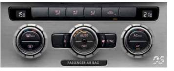
*03* The 2ZONE ELECTRONIC CLIMATE CONTROL with automatic air recirculation features dual zone temperature control for the driver and front passenger, allowing each to select their individual preferred temperature. Standard on all models.
