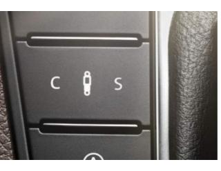
**DYNAMIC CHASSIS CONTROL (DCC)** gives you the choice to select Sport, Comfort or Normal settings for your journey with a touch of a button, and adapts the damping control and shock absorption rate to the road conditions and driving style you require within milliseconds. Standard on 2.0 litre TDI 184 PS models, and optional on all other models.
