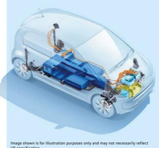
Recuperation is the recovery of energy usually lost when braking. On the e-up! this is achieved by changing the drive motor to generator operation and feeding the resulting current into the vehicle battery, where it is saved for later use. e-up! drivers can choose from four different, easy-to-activate recuperation modes, ranging from maximum delay, achieving optimum brake energy recovery, to minimal delay, achieving less recovery.
