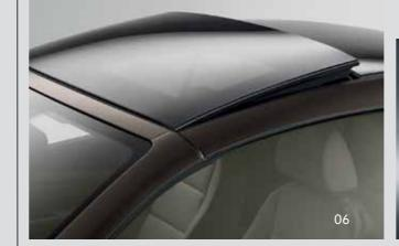
06 The **electric slide/tilt glass sunroof** can be tilted upwards by 35 millimetres, letting light and fresh air into the passenger compartment regardless of the weather. Tinted glass provides protection against the sun, and if you'd like more fresh air, the sunroof slides open towards the rear.
