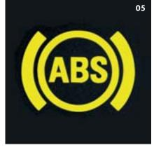
**05** The Anti-lock Braking System (ABS) prevents wheels from locking when braking suddenly and is fitted as standard.
