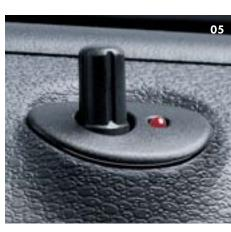
**05** The alarm with interior protection has a monitor that detects movement in the car and, if appropriate, triggers the alarm. Optional on both models.
