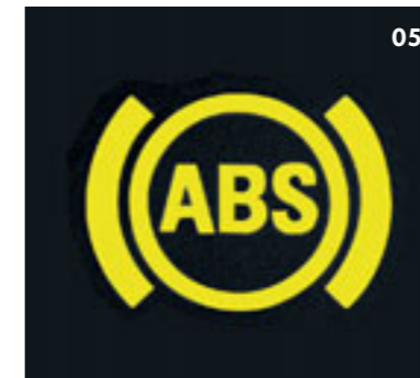
05 The Anti-lock Braking System (ABS) prevents wheels from locking when braking suddenly and is fitted as standard.
