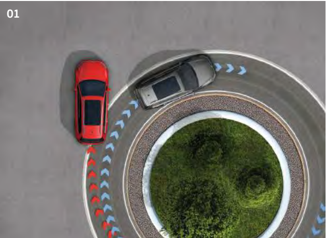
01 // XDS The Golf Estate features XDS, an extension of the well-known Electronic Differential Lock (EDL) function. This is linked to the Electronic Stability Control (ESC) hydraulics and works by applying pressure to the inner front wheel during fast cornering to prevent spinning. The one-sided, precise brake pressure helps to maximise traction, reduce understeer and improve responsiveness, thus making cornering even more accurate. Standard on S, Match Edition, Match BlueMotion Edition, GT and Alltrack models. XDSPlus is standard on GTD and R models.
