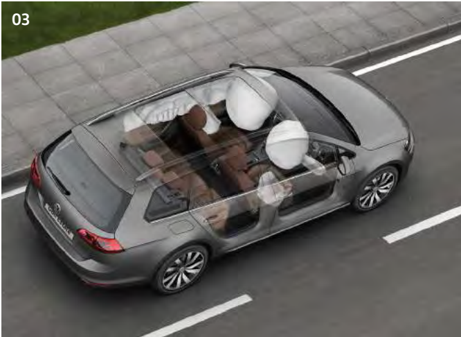
03 // AIRBAG SYSTEM The comprehensive airbag system includes curtain airbags for front and rear passengers, front seat side impact airbags, driver's and front passenger's airbags with passenger's airbag deactivation switch and a driver's knee airbag. Standard on all models. Side airbags and seat belt tensioners for rear passengers are available as an option on all models.
