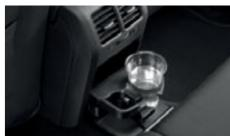
The **front centre armrest** provides additional comfort for the driver, while the rear seat passengers also benefit from two rear air vents and two cup holders. Optional on all S models and standard on all SE and Sportline models.
