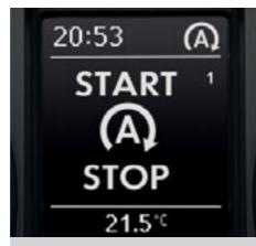
A Start/Stop function\* automatically stops the engine when the vehicle is stationary, in neutral and the clutch released then cleverly restarts it when you depress the clutch to select first gear, saving fuel and reducing emissions.
