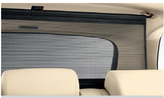
Keep your luggage safely in place with the **retractable net partition.** This option has a two position usage and can be used with the seats upright or when folded flat. Optional on all models.
