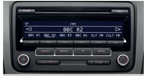
The RCD 310 radio/MP3 compatible CD player features eight speakers with an output of 4 x 20 watts, ensuring a rich sound, and also includes an AUX-in socket for connection to an external multimedia source (e.g. iPod or MP3 player).
