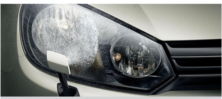
Headlight washers form part of the **Winter pack**, along with heated front seats, a low washer fluid warning light and automatically heated windscreen washer jets. Optional on all models.
