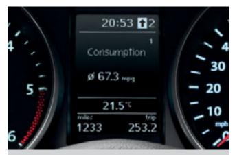
The multifunction computer (Highline) provides useful statistics about your journey, such as exterior temperature, average and current fuel consumption, average speed and estimated distance to refuelling. It also includes a visual gear change recommendation for optimum fuel consumption. Standard on all BlueMotion Technology models.
