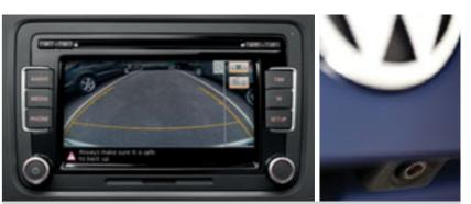
The **rear-view camera** provides a clear view to the rear of your vehicle, transmitting an undistorted live image to your radio display and enabling you to park easily and safely. This also helps when towing a trailer. Optional on all SE and Sportline models.
