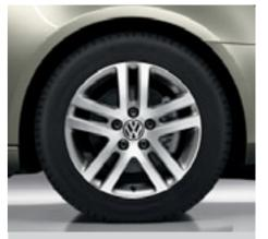
Stylish 16 inch 'Atlanta' alloy wheels with 205/55 R16 tyres and anti-theft wheel bolts provide a distinctive look to the exterior. SE BlueMotion Technology is fitted with 205/55 R16 low rolling resistance tyres as standard.
