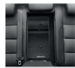
When the rear centre armrest is folded down, it provides a useful **load-through facility**, enabling you to transport skis, snowboards and other long objects easily and conveniently.
