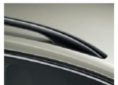
Black roof rails are extremely practical and can be fitted with various carrier systems for transporting bulky items.
