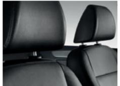
Whiplash-optimised front head restraints are height-adjustable, not only ensuring additional comfort, but also providing effective support for the head and spine in the event of a collision.
