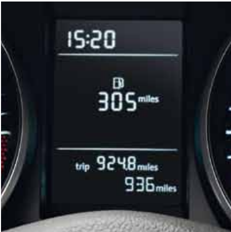
The multifunction computer (Midline) can be operated easily, and provides useful information such as average and current fuel consumption, journey time, outside temperature and range left in the fuel tank.
