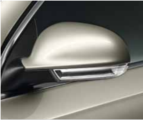
The electrically heated and adjustable body-coloured door mirrors with integrated indicators not only complement the body styling, but are also highly visible to other road users.
