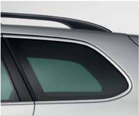
Heat insulating tinted rear windows from the B pillar back are 65% light absorbing, helping reduce exposure to the sun’s rays, whilst giving your Golf Estate a sporty look.
