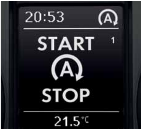
A Start/Stop function* automatically stops the engine when the vehicle is stationary, in neutral and the clutch released then cleverly restarts it when you depress the clutch to select first gear, saving fuel and reducing emissions.
