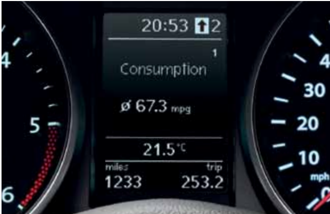
The multifunction computer (Highline) provides useful statistics about your journey, such as exterior temperature, average and current fuel consumption, average speed and estimated distance to refuelling. It also includes a visual gear change recommendation for optimum fuel consumption. Standard on all BlueMotion Technology models.
