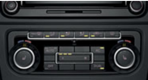
The 2Zone electronic climate control with automatic air recirculation system features dual zone temperature control for the driver and front passenger, enabling each to select their individually preferred temperature.
