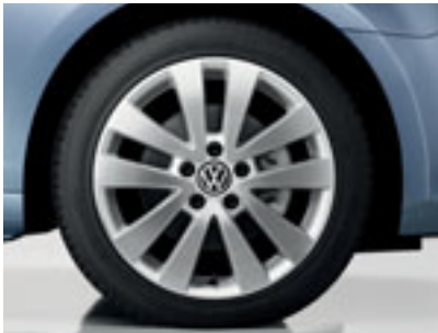
‘Seattle’ 7J x 17 light alloy wheels with 225/45 R17 tyres. Optional on SE and GT models. Please note: SE models also include lowered sports suspension.
