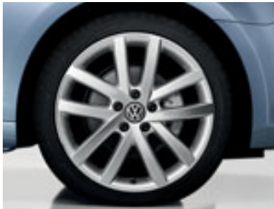
‘Vancouver’ 7½J x 18 light alloy wheels with 225/40 R18 tyres. Optional on GT and GTD models.
