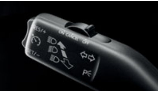
At speeds of over 19 mph, cruise control keeps your selected speed constant, enabling you to relax on longer journeys, without having to keep an eye on your speedometer.
