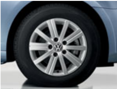
‘Wellington’ 6½J x 15 light alloy wheels with 195/65 R15 tyres. Standard on BlueMotion and optional on S models. Please note: BlueMotion models are fitted with 195/65 R15 low rolling resistance tyres.
