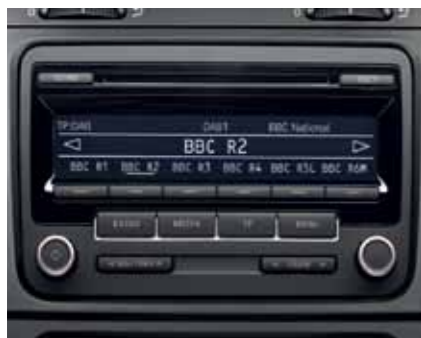
The RCD 310 DAB radio/MP3 compatible CD player features eight speakers with an output of 4 x 20 watts. It also features an AUX-in socket for connection to an external multimedia source (e.g. iPod or MP3 player).
