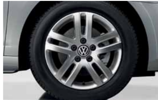
16 inch 'Cleveland' alloy wheels with low rolling resistance tyres, for the GT BlueMotion Technology model, not only look good, but they also help to reduce fuel consumption.
