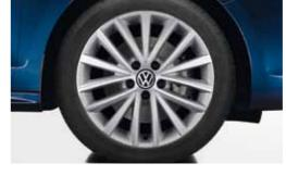
**'Porto'** 7J x 17 alloy wheels provide secure handling and roadholding, with 225/45 R17 tyres and anti-theft wheel bolts.
