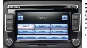
The RCD 510 touch-screen radio/dashmounted MP3 compatible six CD autochanger features a large 6½ inch colour display, with intuitive menu navigation and touch-screen operation. It also features an AUX-in socket for connection to an external multimedia source such as iPod or MP3 player and an SD card slot.
