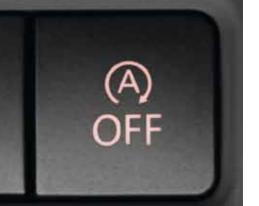
The **Start/Stop function** turns off the engine when the vehicle is stationary, in neutral and the clutch disengaged, and this is notified via a symbol on the multifunction computer display. This occurs when the engine is idle, such as at traffic lights, then restarts when you put the vehicle back in gear, thereby saving fuel.
