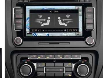
**2Zone electronic climate control with automatic air recirculation,** controls the temperature electronically and divides the interior into two different climate zones, enabling the driver and front passenger to adjust the temperature, air supply and distribution to suit their individual preference.
