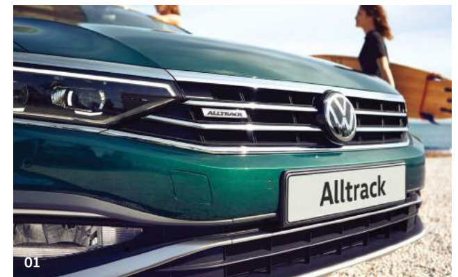
01 The stylish front design is sporty and eye-catching with LED headlights blending seamlessly into the new chrome radiator grille complete with the exclusive 'Alltrack' logo. Striking 'Gloss Black' surrounds featuring integrated fog lights with static cornering function complete the look. Image shown features optional 'IQ. Light' LED matrix headlights and metallic paint.
