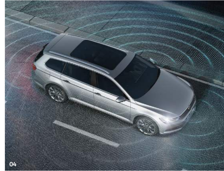
04 Area view . Four cameras located in the boot lid/tailgate, door mirrors and radiator grille, each with an aperture angle of over 180 degrees, provides a 360-degree view around the Passat helping you manoeuvre in confidence in any direction. From the display menu, the driver can select the camera views; front, rear, side or bird's-eye view, on either full or split-screen, displayed on the Passat's infotainment system. Standard on GTE Advance and optional on SE Business models and above. Not in conjunction with rear-view camera. Model shown features optional metallic paint.
