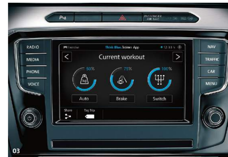
03 The Car-Net 'App-Connect' combines functionality of Apple 'CarPlay', Google 'Android Auto' and 'MirrorLink™' allowing 'mirroring' of a smartphone display on the infotainment touch-screen via USB connection. Only operable in conjunction with compatible smartphones including iPhone 5, 6 and 7. Volkswagen apps such as 'Think Blue Trainer', 'Shared Audio', 'Drive & Track' or 'My Guide' can help to make your journey more pleasant and interesting, providing useful tips about handling your car, parking opportunities and even where to find the closest café. Volkswagen apps are only available with compatible smartphones. Please consult www.volkswagen.co.uk to check smartphone compatibility. Usage of certified apps only while driving. Standard on GTE Advance and optional on all other models. Car-Net 'App-Connect' is included with the optional Discover Navigation Pro touch-screen navigation/DVD radio system. Discover Navigation Pro radio system is standard on GTE Advance models.
