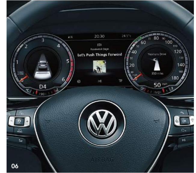
05 – 06 The Active Info Display 1 . Ideal for those who love the latest technology, providing a system that can be tailored to suit your specific preferences. A fully configurable, interactive, 12.3 inch high resolution TFT dash display replaces the standard instrument cluster, displaying vehicle data and information on your dashboard. A choice of five different modes enables you to customise the screen as you wish, showing large or small dials as you prefer, with a number of items displayed behind. In navigation mode, for example, you can move the speedometer and rev counter to the edge of the display, creating more space for the navigational map. If you wish, you can include driving, navigation and assistance functions within the graphics of the speedometer. As the Active Info Display is linked to all other assistance systems in the vehicle, any data shown in the centre console of the infotainment system, such as phone numbers or compatible cover art, can also be displayed on the dash, conveniently placed directly within the driver's optimum field of vision. Standard on GT, R-Line and GTE Advance and optional on SE Business, GTE and Alltrack models.
