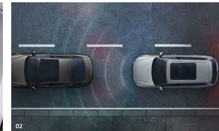
02 Adaptive Cruise Control (ACC) , including Front Assist radar sensor controlled distance monitoring system, City emergency braking system, cruise control and speed limiter offers you intelligent control of your driving speed by automatically adjusting acceleration and braking. Whether around town or on the motorway, the system will adjust your speed to that of the vehicle in front, keep your specified distance, warn if you are approaching too fast and, in an emergency situation, generate enough braking force to try to reduce the severity of a collision or possibly even prevent the collision entirely. Image shown is for illustration purposes only and may not necessarily reflect UK specification.
