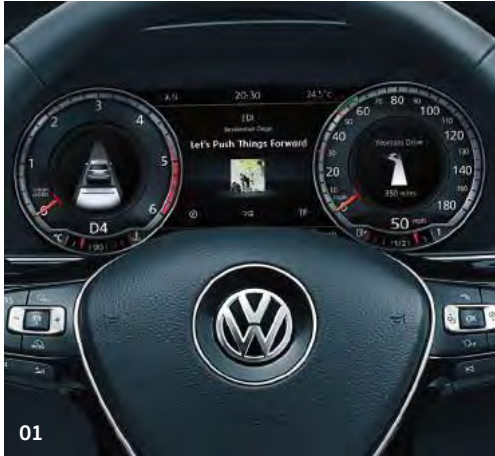
01 The innovative Active Info Display ingeniously displays all instrumentation in a fully interactive virtual format, with high quality graphics on a large 12.3 inch screen.
