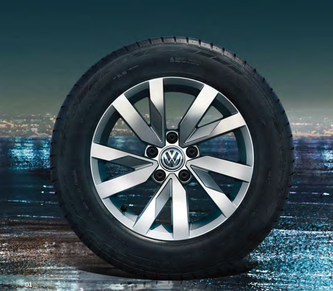
01 'Aragon' 6½J x 16" alloy wheels with 215/60 R16 low rolling resistance tyres and anti-theft wheel bolts. Standard on S models.
