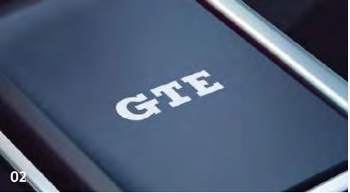
02 The Driver profile selection includes ‘GTE’ mode, which activates its sportier side. At the touch of the GTE button, the electric and petrol motors combine to deliver 218 PS and a top speed of 140mph where the law permits. The steering wheel also becomes more responsive and the chassis firms up, the DSG gearbox changes gear quicker, keeping in the lower gears ready to accelerate on demand.
