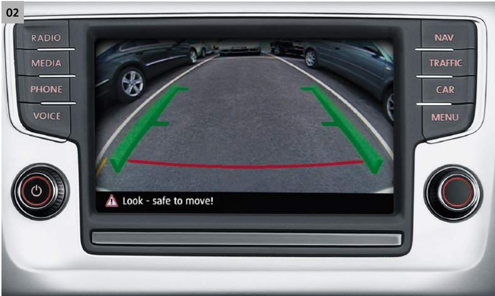
02 REAR-VIEW CAMERA The rear-view reversing camera makes parking easier by emitting audible signals and displaying the area behind the vehicle on the audio system or navigation system's display. Auxiliary lines help you navigate safely into parking spaces, and thanks to the high resolution display, even small obstacles such as kerbs are clearly visible. Optional on all models. Image shown features optional Discover Navigation touch-screen navigation/radio system.
