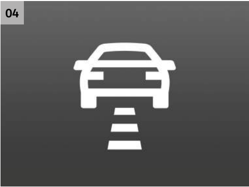
04 ADAPTIVE CRUISE CONTROL (ACC) including Front Assist radar sensor controlled distance monitoring system, City emergency braking system and cruise control. ACC offers you intelligent control of your driving speed by automatically adjusting acceleration and braking. The system will adjust your speed to that of the vehicle in front, keep your specified distance, warn if you are approaching too fast and, in an emergency situation, generate enough braking force to reduce the severity of a collision or even prevent the collision entirely. Optional on SE, SE Design, SEL, BlueMotion and BlueGT models.
