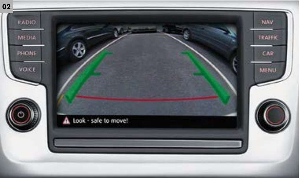
02 REAR-VIEW CAMERA The rear-view reversing camera makes parking easier by emitting audible signals and displaying the area behind the vehicle on the audio system or navigation system’s display. Auxiliary lines help you navigate safely into parking spaces, and thanks to the high resolution display, even small obstacles such as kerbs are clearly visible. Optional on all models. Image shown features optional Discover Navigation Pro touch-screen navigation/radio system.
