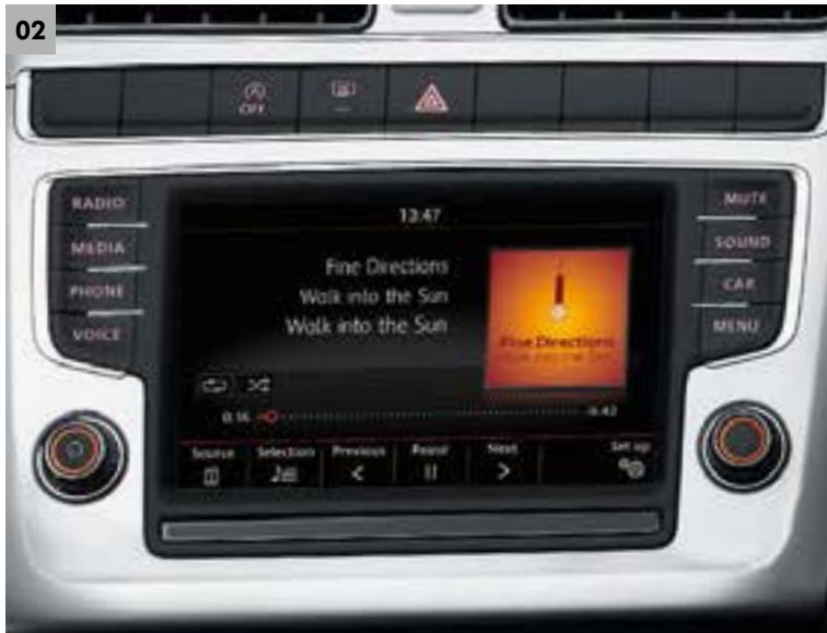
02 COMPOSITION MEDIA SYSTEM 6.5 inch colour touch-screen with proximity sensor, an MDI (Multi Device Interface) via USB connection for connectivity to an external multimedia source – including Apple products, title and cover art display, SMS functionality allowing you to read, compose and send SMS messages using touch-screen display and glovebox-mounted CD player. It also includes Think Blue. Trainer. – which provides driver tips and journey analysis for more ecological driving and Bluetooth telephone and audio connection for two compatible devices 2 at the same time. Standard on SE models and above.
