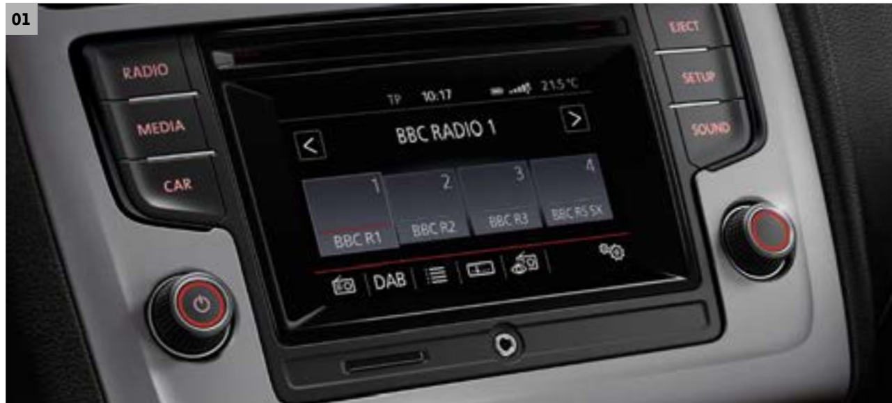
01 COMPOSITION COLOUR SYSTEM with 5 inch colour touch-screen, an AUX-in socket for connection to an external multimedia source, such as an iPod or MP3 player, a DAB digital radio receiver, dash-mounted single CD player, SD card reader, music playback from MP3, WMA and AAC files, USB connectivity 1 and six speakers. It also features Bluetooth telephone and audio connection for compatible devices 2 and you can also connect two devices at the same time. Standard on S and S A/C models.
