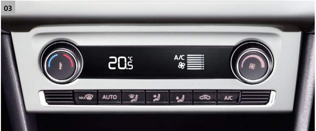
03 ELECTRONIC CLIMATE CONTROL AIR CONDITIONING provides your required cabin temperature quickly and effectively, while maintaining your selected temperature. Optional on S A/C models and above.
