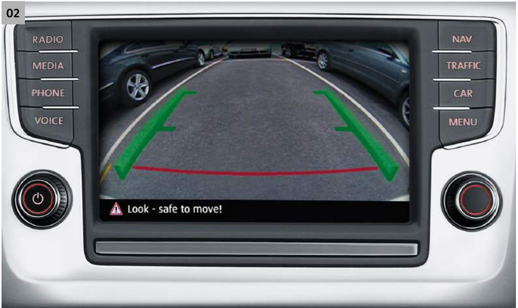
02 REAR-VIEW CAMERA The rear-view reversing camera makes parking easier by emitting audible signals and displaying the area behind the vehicle on the audio or navigation system’s display. Auxiliary lines help you navigate more easily into parking spaces, and thanks to the high resolution display, even small obstacles such as kerbs are clearly visible. Optional on SE models and above.
