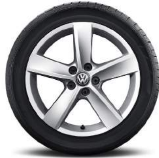
'RIVAZZA' 7J x 16 inch alloy wheels with 215/45 R16 tyres. Standard on SEL models.
