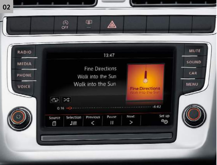
02 COMPOSITION MEDIA SYSTEM 6.5 inch colour touch-screen with proximity sensor, an MDI (Multi Device Interface) via USB connection for connectivity to an external multimedia source (compatible products only), title and cover art display, glovebox-mounted CD player and six speakers. The media system also includes 'Think Blue. Trainer.' 3 – providing driver tips and journey analysis, Bluetooth telephone and audio connection for two compatible devices 2 at the same time and SMS functionality, allowing you to read, compose and send SMS messages using the touch-screen display when your Polo is stationary (compatible Android smartphones only). Standard on Match models and above.
