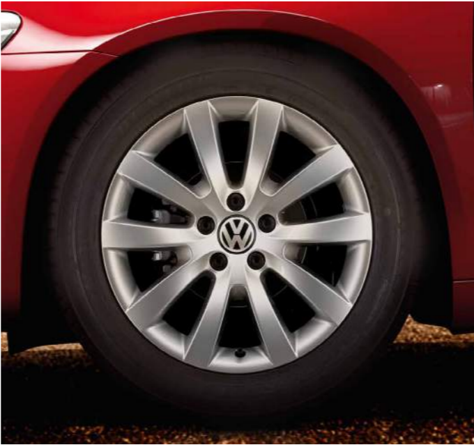
'Long Beach' 7J x 17" alloy wheels with 205/50 R17 tyres are an eye-catching addition to the exterior of the Scirocco. Model shown features optional non-metallic signature paint.
