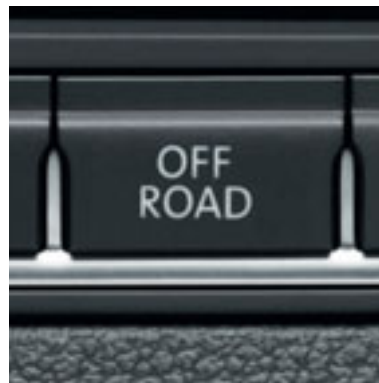
The off-road mode includes hill descent assist and ABSPlus adjusted to suit loose ground.
