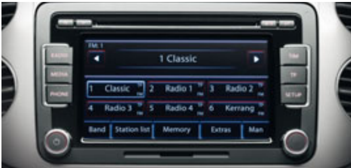
Dynamic: The RCD 510 touch-screen radio/dash-mounted MP3 compatible six CD autochanger with eight speakers and AUX-in socket for connection to an external multimedia source (e.g. iPod and MP3 player).
