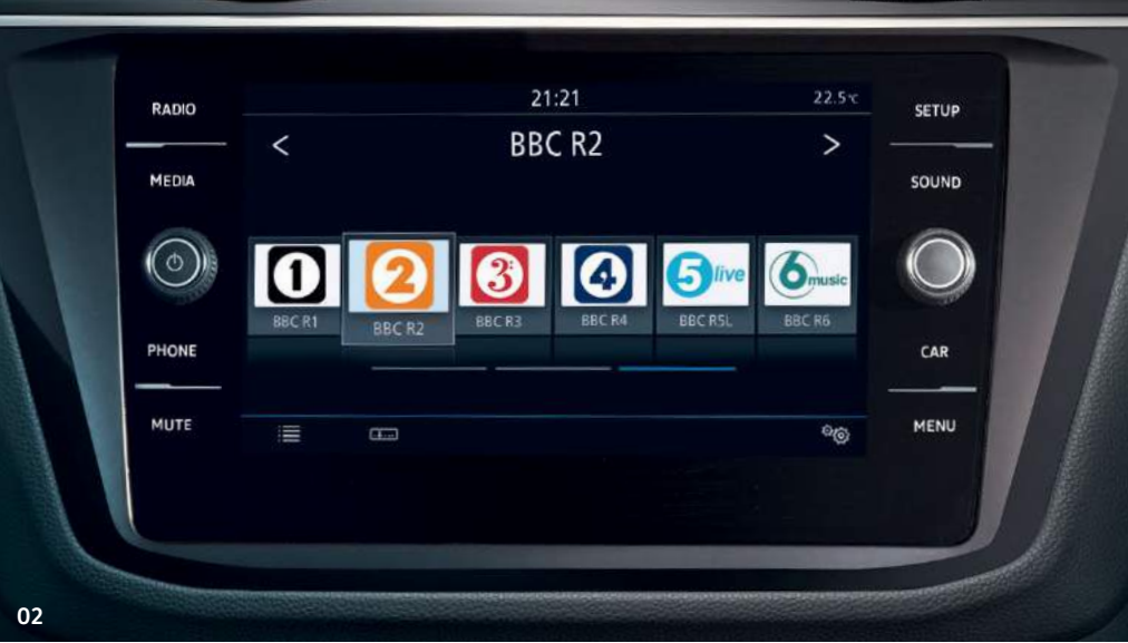
02 The Composition Media system is equipped with an impressive 8.0 inch colour touch-screen with proximity sensor that recognises in advance your intention to touch the screen and automatically magnifies the display mode. Features also include DAB digital radio receiver, CD player, USB connection for compatible products and SD card reader. The media system also includes Bluetooth telephone and audio connection for compatible devices², simultaneous pairing of two compatible mobile devices, SMS functionality – allowing you to read, compose and send SMS messages using the touch-screen display to a compatible Android smartphone (while the vehicle is stationary), title and compatible cover art display and facilitates music playback from MP3, WMA and AAC files through eight speakers, front and rear. Finally, car information display and ‘Think Blue. Trainer.’ – provide journey analysis and driver tips during your journey. Standard on S and SE models.
