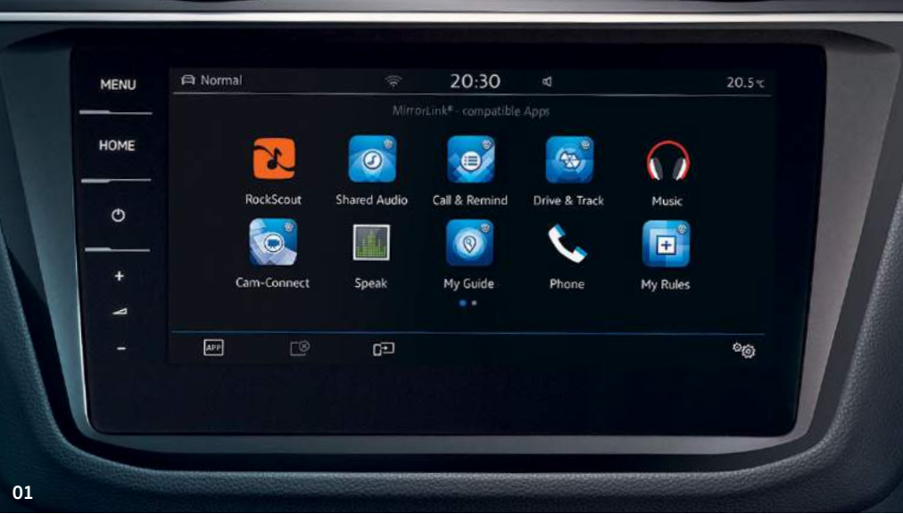
01 Depending on which smartphone you have, you can connect Car-Net ‘App-Connect’ 1 via one of three interfaces: Apple ‘CarPlay’, Google ‘Android Auto’ or ‘MirrorLink’™, allowing your smartphone display to be ‘mirrored’ on the infotainment touch-screen via USB connection and giving access to your favourite smartphone functions, such as music, messages, phone and news. Volkswagen apps such as ‘Think Blue. Trainer’, ‘Shared Audio’, ‘Drive & Track’ or ‘My Guide’ can help to make your journey more pleasant and interesting by providing useful tips about handling your car, parking opportunities and even where to find the closest café. Volkswagen Apps are only available with compatible smartphones. Please consult www.volkswagen.co.uk to check smartphone compatibility. Usage of certified apps only while driving. Standard on SE models and above. Optional on S models. Image shown features optional Discover Navigation Pro touchscreen navigation/DVD radio system.
