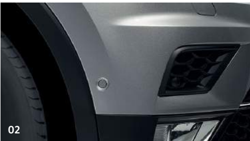
02 The Park Assist system not only makes parallel parking easier, but also helps you reverse park into a space at 90 degrees to the kerb. Using ultrasonic sensors, Park Assist will detect a parking space large enough for either bay or parallel parking. Once the vehicle is in reverse, all the driver has to do is operate the accelerator and brake, and keep a lookout, while the Tiguan steers itself into its chosen space. Optional on SE models and above. Park Assist including parking sensors, front and rear is available on S models.
