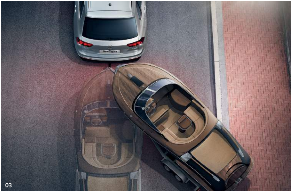
03 The new Tiguan effortlessly tows a trailer or caravan and, depending on your choice of engine, can tow up to a maximum weight of 2.5 tons. Trailer Assist including Park Assist and rear-view camera helps you reverse more easily and accurately with a trailer or caravan attached. The optical display visualises actual and possible steering angles in the instrument cluster. Reverse steering is automatic, with direction controlled via the mirror adjustment switch which acts as a joystick, while the driver controls the pedals and keeps a good look out. Only in conjunction with the optional swivelling towbar. Optional on SE models and above.
