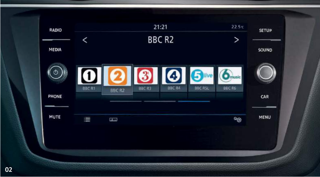
02 The Composition Media infotainment system is equipped with an impressive 8.0 inch colour touch-screen with proximity sensor that recognises in advance your intention to touch the screen and automatically magnifies the display mode. Features also include DAB digital radio receiver, CD player, USB connection for compatible products and SD card reader. The media system also includes Bluetooth telephone and audio connection for compatible devices 2 , simultaneous pairing of two compatible mobile devices, SMS functionality – allowing you to read, compose and send SMS messages using the touch-screen display to a compatible Android smartphone (while the vehicle is stationary), title and compatible cover art display and facilitates music playback from MP3, WMA and AAC files through eight speakers, front and rear. Finally, car information display and ‘Think Blue. Trainer.’ – provide journey analysis and driver tips during your journey. Standard on S models.
