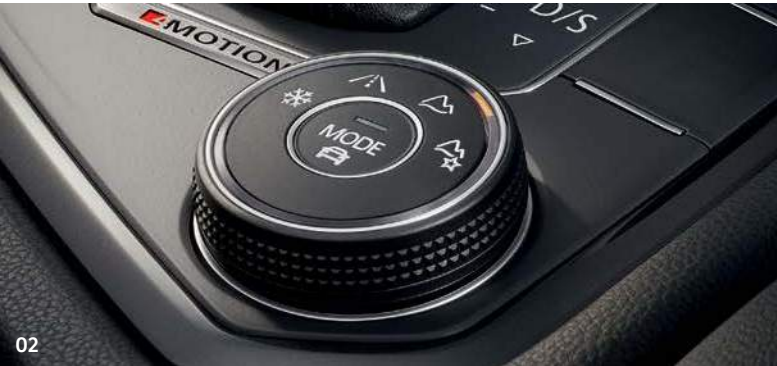
02 All 4MOTION models feature 4MOTION Active Control which allows you to adapt your Tiguan to suit the weather and road conditions ahead. Choose from four driving modes including On road, Off-road, Off-road Individual and Snow, enabling you to find the optimum choice of driving mode wherever your adventures may take you. Standard on all 4MOTION models. Image shown features optional 'Vienna' leather upholstery.
