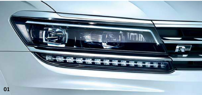
01 Daytime running lights feature LED technology for greater visibility, and fit flush with the LED headlights with Dynamic Light Assist, enhancing the Tiguan's sporty look. Standard on SEL and R-Line Tech. Optional on Match models. Model shown features optional premium signature paint.
