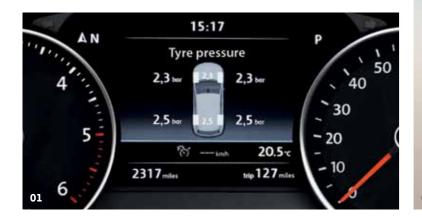
**01** The electronic tyre pressure monitoring system keeps you informed about the air pressure of each tyre via the multifunction display, warning you of any changes. This enables you to maintain optimum tyre pressure, increasing the lifespan of the tyres and reducing fuel consumption. Standard on all models.
