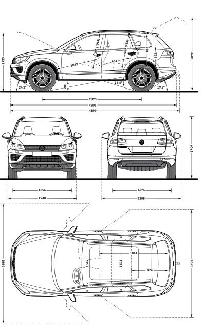
All figures in millimetres. On illustrations, where arrows and figures are shown inside of the vehicle, the measurements are for interior dimensions. Where arrows and figures are shown outside of the vehicle, the measurements are for exterior dimensions.
