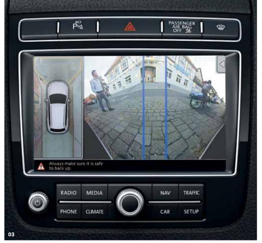
**04** Area View's reversing camera provides a view of the area behind your Touareg, transmitting an image direct to the RNS 850 Connect touch-screen navigation/radio system's display. Superimposed lines show the path you should take when reversing, ensuring you avoid obstacles below eye level. Optional on all models as part of Area View.
