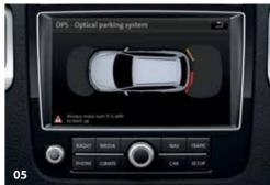
05 Parking sensors issue an optical and audible warning as soon as your vehicle approaches an object to the front or rear when manoeuvring into a parking space. Standard on all models.
