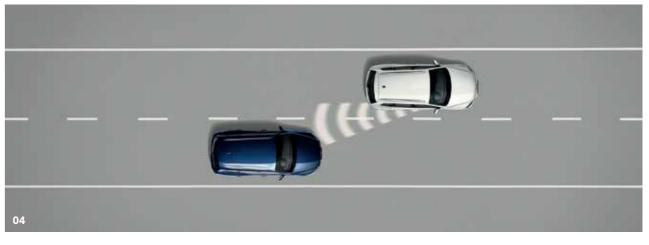
**03 Automatic Post-Collision Braking System** starts the brake operation after impact to help avoid further collisions. Standard on all models.
