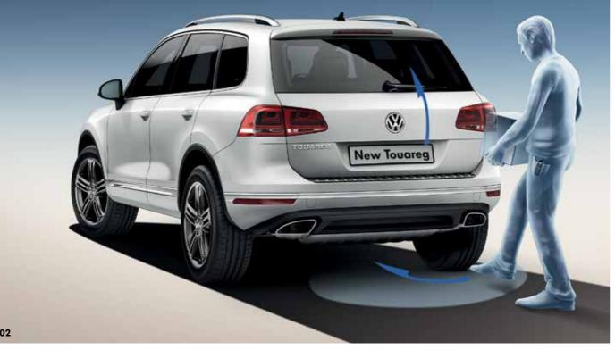
02 The hands free tailgate opening function enables you to open the tailgate without having to make contact with your Touareg. A small foot movement triggers sensors at the vehicle's rear. Hands free tailgate opening is a function of the optional Keyless entry/keyless start and full electric tailgate operation. Optional on SE and Escape models.
