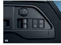
**08** The **control panel** in the boot automatically releases the rear seat backrest and the optional towbar, and also lowers the rear of the vehicle for easy loading and unloading.
