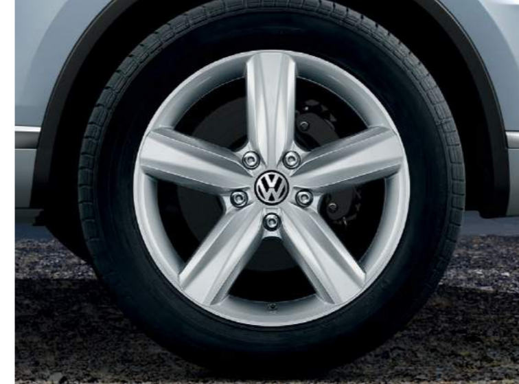
SE 'Girona' 8½J x 19 inch alloy wheels 265/50 R19 110W low rolling resistance tyres and anti-theft wheel bolts.
