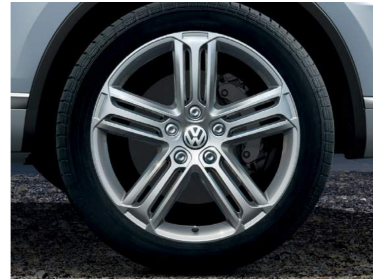
SE RL 'Talladega' 9J x 20 inch alloy wheels 275/45 R20 110W low rolling resistance tyres and anti-theft wheel bolts. No cost option on R-Line models.
