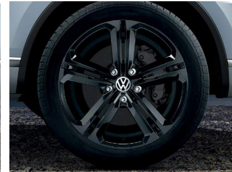
RL RLP 'Mallory Black' 9J x 20 inch alloy wheels 275/45 R20 110W low rolling resistance tyres and anti-theft wheel bolts. No cost option on R-Line Plus models.
