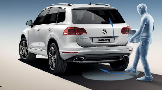
02 The hands free tailgate opening function enables you to open the tailgate without having to make contact with your Touareg as long as you have the key in your possession. A small foot movement triggers sensors at the vehicle's rear and the rear tailgate will open out. Hands free tailgate opening is a function of the optional keyless entry/keyless start and full electric tailgate operation. Optional on SE models.
