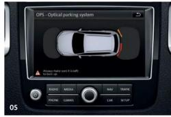
05 Parking sensors, ultrasonic front and rear alert you with an optical and audible warning as soon as your vehicle approaches an object to the front or rear when manoeuvring into a parking space. A visual representation of how close the front or rear of the vehicle is to an object will also be displayed on the vehicle's radio system display. Standard on all models.
