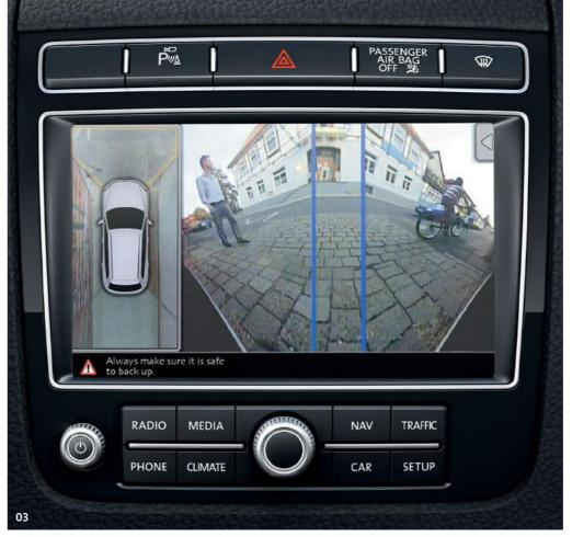
04 Area view's reversing camera provides a view of the area behind your Touareg, transmitting an image direct to the RNS 850 Connect touch-screen navigation/DAB radio system's display. Superimposed lines advise you of the path you should take when reversing, ensuring you avoid obstacles below eye level. Standard on R-Line Plus models and optional on all other models as part of Area view.
