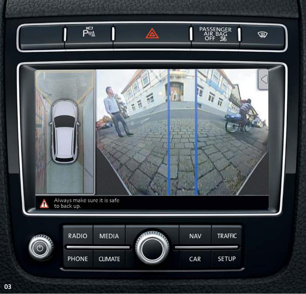
03 Area view's front, rear and side cameras provide a 360 degree exterior view around your Touareg transmitted to the RNS 850 Connect touch-screen navigation/DAB radio system's display, providing a bird's-eye view to the front and enabling you to see around left and right hand corners to an angle of over 90 degrees. Standard on R-Line Plus models and optional on all other models.
