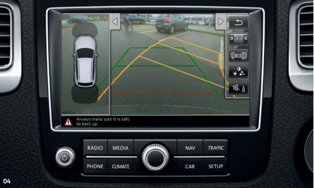
05 Parking sensors alert you with an optical and audible warning as soon as your vehicle approaches an object to the front or rear when manoeuvring into a parking space. A visual representation of how close the front or rear of the vehicle is to an object will also be displayed on the vehicle's radio system display. Standard on all models.
