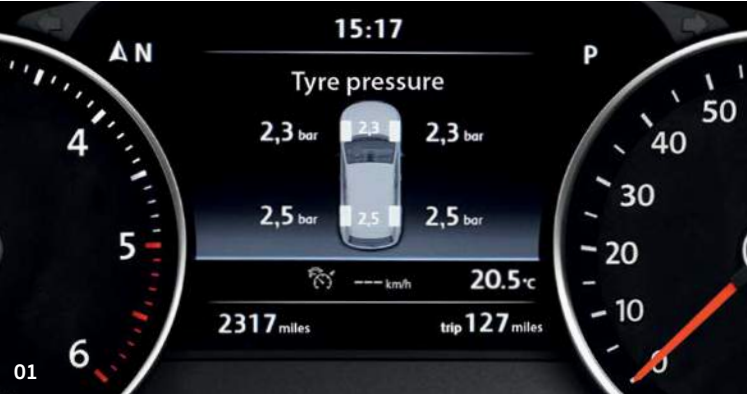
01 The electronic tyre pressure monitoring system keeps you informed about the air pressure of each tyre via the multifunction display, warning you of any changes. This enables you to maintain optimum tyre pressure, thereby increasing the lifespan of the tyres. Standard on all models.
