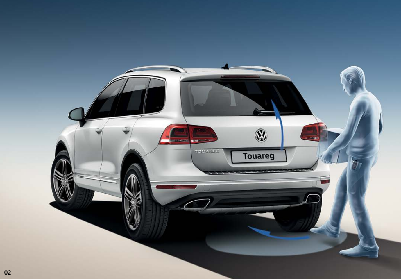
02 The hands free tailgate opening function enables you to open the tailgate without having to make contact with your Touareg as long as you have the key in your possession. A small foot movement triggers sensors at the vehicle's rear and the rear tailgate will open out. Hands free tailgate opening is a function of the optional keyless entry/keyless start and full electric tailgate operation . Optional on SE models.
