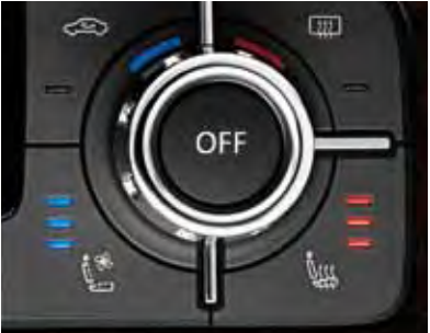
The climate function for the driver’s and passenger’s front comfort seats regulates the ventilation of the seat surfaces, backrests and side bolsters, and are equipped with three different settings to suit your individual requirements.
