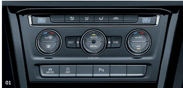
01-02 The climate control – 3Zone electronic air conditioning system allows the driver, front passenger and those seated in the 2nd row to set their own desired temperature, independently of one another. This advanced air conditioning system also features a 'gentle' climate option, making steamed-up windows a thing of the past, while the biogenic filter keeps out pollens and allergens, ensuring consistent air quality throughout the passenger compartment. Standard on SEL and R-Line and optional on all other models.
