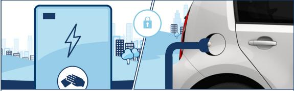
2. You swipe your smart card on the unit's reader and then you can plug the DC charger cable into your car. The larger DC units have a cable that connects to your car so it means you don't need to use your own cables. When you lock your car doors this also locks the cables so charging can begin.
