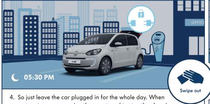
you return to your car swipe the smart card to stop the charging and unlock the cables at both ends.
