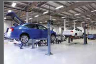
A PDI (pre-delivery inspection) centre runs checks for faults that may have developed post-production, fits number plates, tests tyre pressures, and so on.
